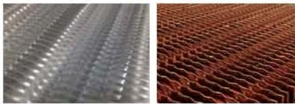
Before Coated After Coated & Curing
